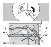
After positioning the inlet hose, be sure to tighten the ring nut again to prevent leaks.
